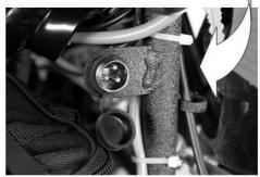
Align the groove (Poka-Yoke) of the charger's 3 pins plug into the ATV's charger connector.
