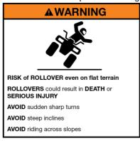
CROSSING HILLSIDES Driving on a sidehill is not recommended. Improper procedure could cause loss of control or overturn. Avoid crossing the side of any hill unless absolutely necessary. If crossing a hillside is unavoidable, always follow proper procedures as described in the owner's manual. Never attempt to turn the ATV around on any hill until you've mastered the turning technique (on level ground)
