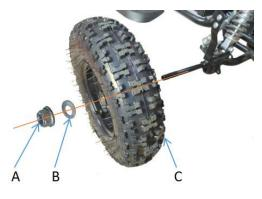
1. Put the front wheel suspension (B) into the front swing arm joint, align the bearing hole to the joint upper and bottom hole
