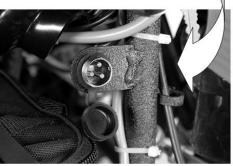
Align the groove (Poka-Yoke) of the charger's 3 pins plug into the ATV's charger connector. Tighten the plug to secure the contact.
